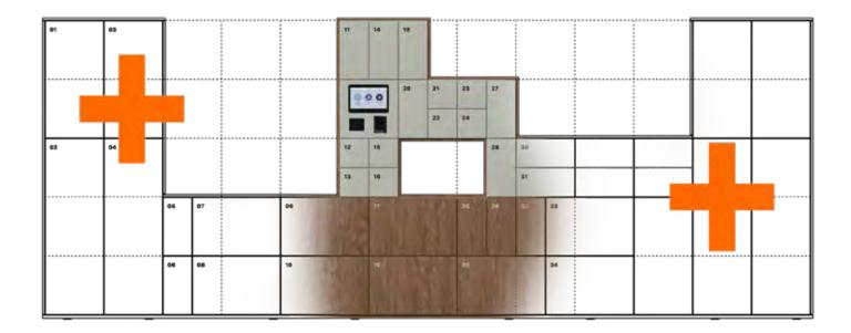
OfficeLine systems are configured from individual modules in a clearly defined grid. The modules are available in different widths (1/2, 1, 1 1/2) and heights (1, 2 or 3). In addition, various compartment divisions can be planned. These gradations allow the OfficeLine to be adapted in a versatile way to the respective installation locations and types of use.
